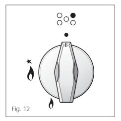
To turn the burner off, fully rotate the knob clockwise to the off position: ●.
